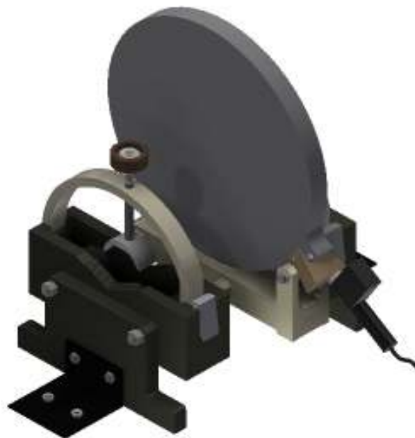
Fig. 12 Assembling between the thermoplastic materials butt fusion welding machine and the electric hob.
