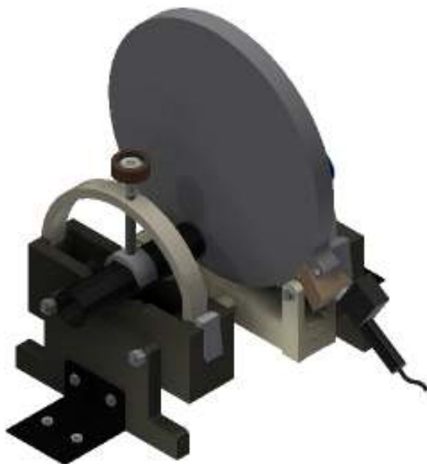
Fig. 13 The CAD model of the thermoplastic materials butt fusion welding machine.
