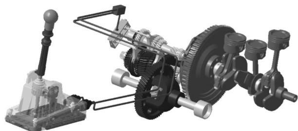
Fig 33. Gearshift-gearbox assembly.
