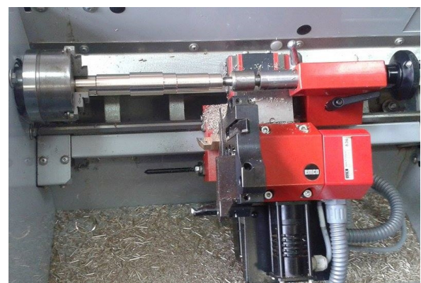
Fig. 2b The straight shaft machined on EMCO CONCEPT TURN 55.
