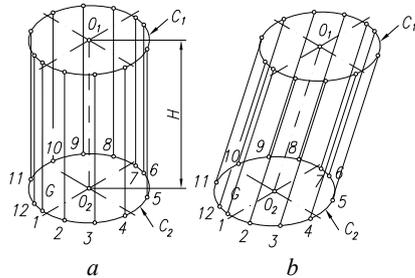
**Fig. 8** Cylinder with extensible generatrix.
