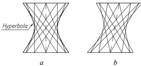
**Fig. 9** Cylinder turned into hyperboloid.
