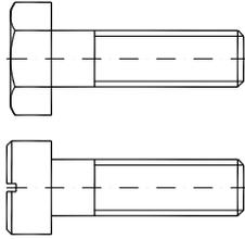
Fig. 3 The screws with different heads.
