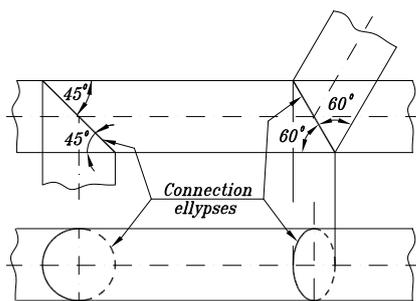
Fig. 15 The banister made of bars or pipes.
