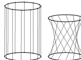
**Fig. 11** Cylinder with inextensible generatrix.
