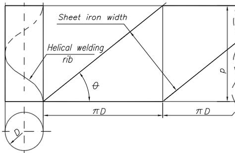
Fig. 13 Cylindrical pipe with great diameter.
