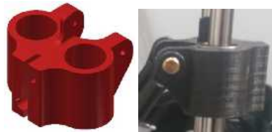
Fig. 11 Bearing fixing system: virtual model (a); physical model (b).
