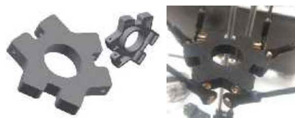
Fig. 12 Holder: virtual model (a); physical model (b)
