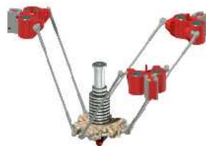
Fig. 13 Guidance-support-cooler system assembly
