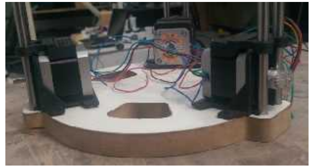
Fig. 19 Lower plate- stepper assembly – physical model
