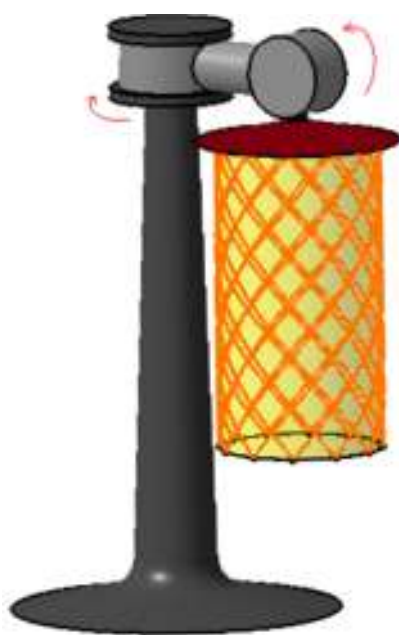
Fig. 9 Lighting body generated by cylindrical helices
