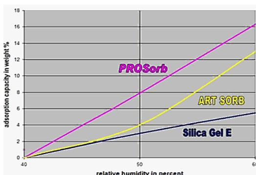
Figure 4 Adsorption capacity in the humidity range 40-60%.
