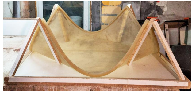
Figure 17 Placing the mold to make the conoid.
