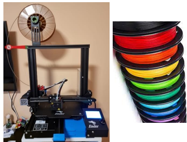
Figure 18 Equipment and printing accessories: a – Creality Ender 3 Pro printer ; b – PLA filaments .
