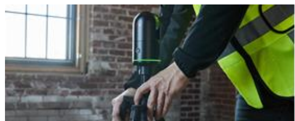
Figure 3 The equipment used Leica BLK360 Imaging Laser Scanner (Source: [14]).
