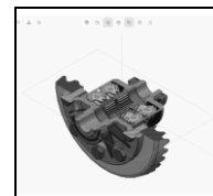
Figure 3 Axonometric section through a gear assembly
