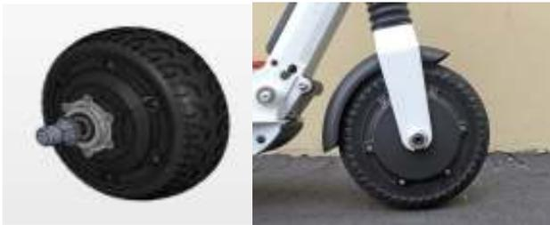
Fig. 7 Hub-centric motor design (left), front wheel drive scooter (right).
