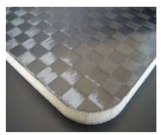
Fig. 6 Sandwich Composite Cut Out [9].
