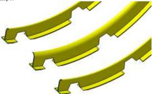
Fig. 5 Frames positioned for assembly.
