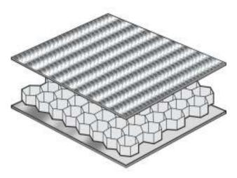
Fig. 2 Honeycomb Composite [8].
